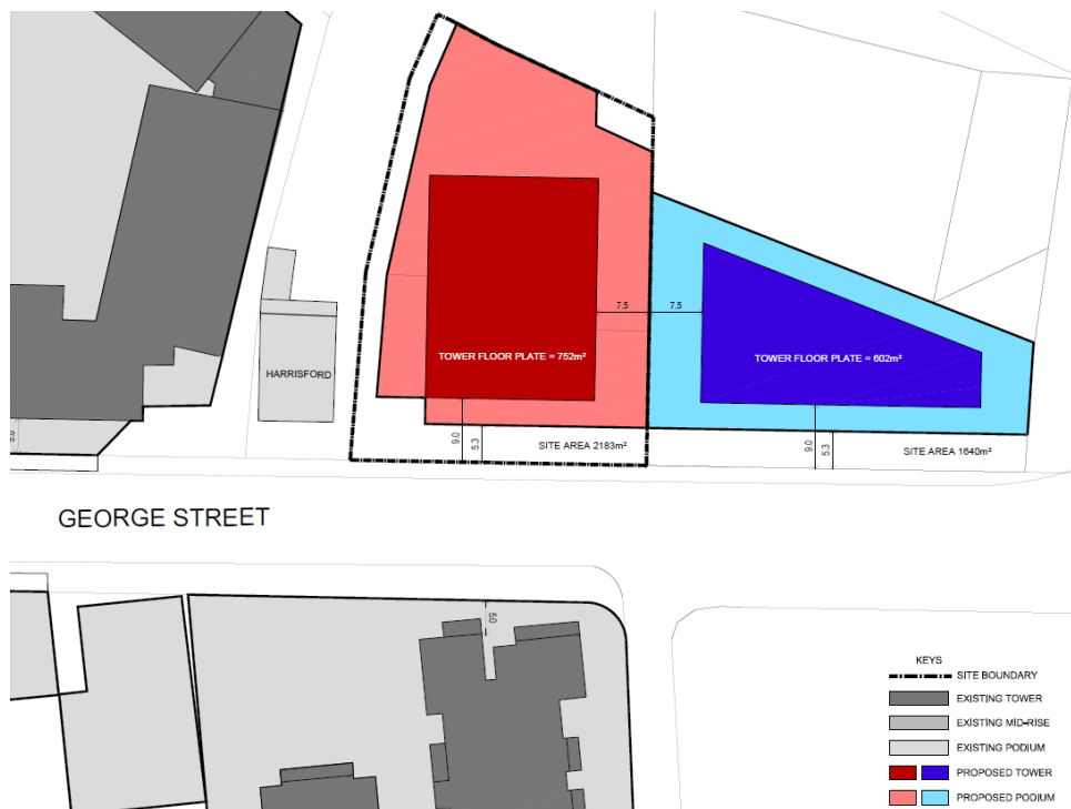
Figure 6: Option 2B – height 120m (38 storeys), FSR 10:1 and tower floor plate 752sqm
